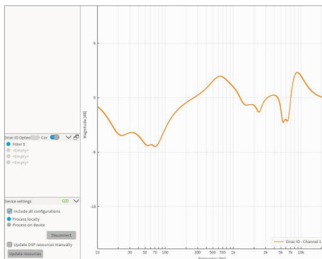
Automatically optimized speaker correction filter response
